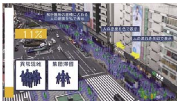
The crowd behavior analysis technology enables to perform highly precise analyses and issues an alert if predetermined threshold levels are exceeded. Without overlooking, initial response can be delivered timely.
