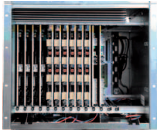
Control and Switching Module
